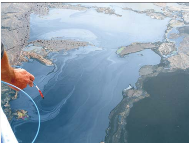
Capturing absorption spectra with a fibre optic probe.
