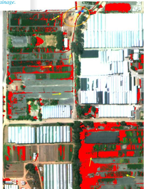
*Multispectral image overlaid with irrigation overflow patterns extracted from thermal IR data.*
