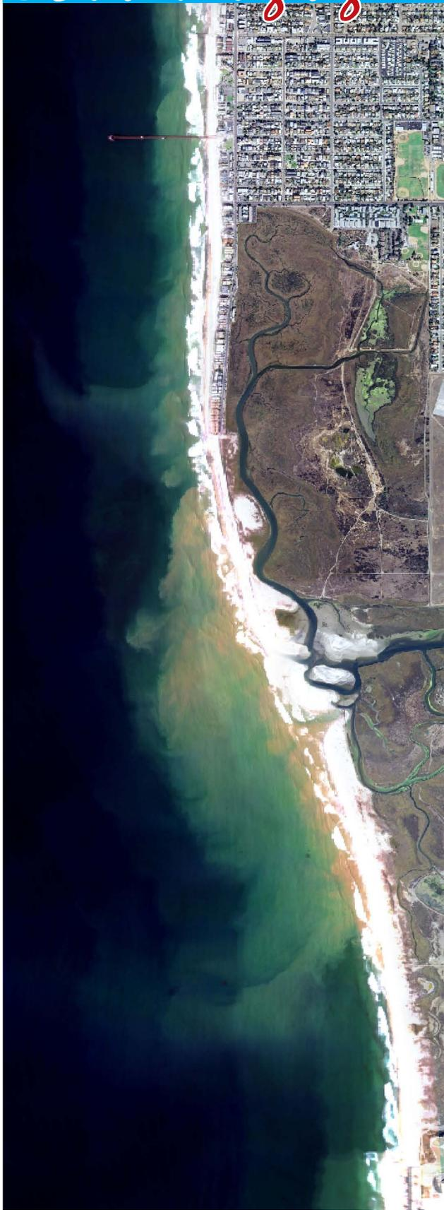
*DMSC multispectral image of the sand replenishment experiment.*
