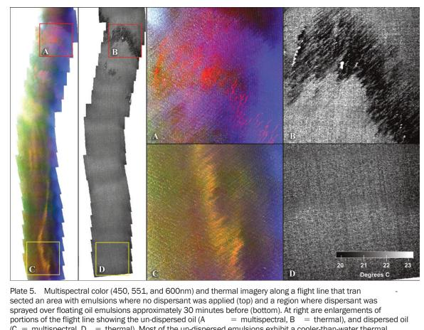
portions of the flight line showing the un-dispersed oil (A = multispectral, B = thermal), and dispersed oil (C = multispectral, D = thermal). Most of the un-dispersed emulsions exhibit a cooler-than-water thermal signature (thinner), with a few smaller areas appearing warmer (thick). The dispersed oil had likely sunk into the water column and is thus no longer discernible in the thermal data.
